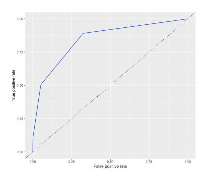
The true positive rate and false positive rate for a tree classifier with cutpoint 0.5.
